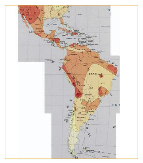
Figure 11. Annual solar radiation map for LAC (kWh/m²/day).
